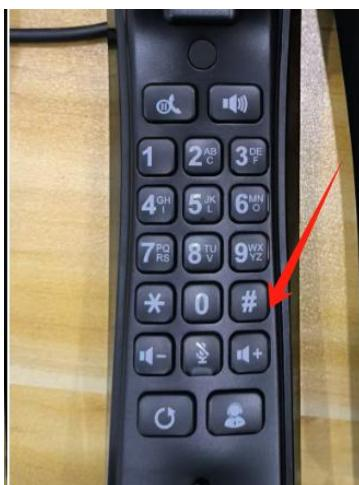
**Without DHCP, unable to get a IP.** Dialing this code, '#\*100', to switch to static IP. The static IP: 192.168.1.128.
