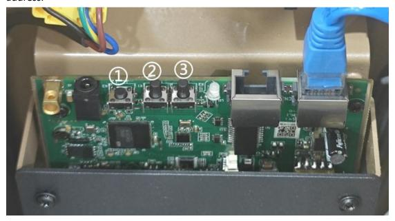
Long press button ① for factory reset, Do not operate unless necessary.
