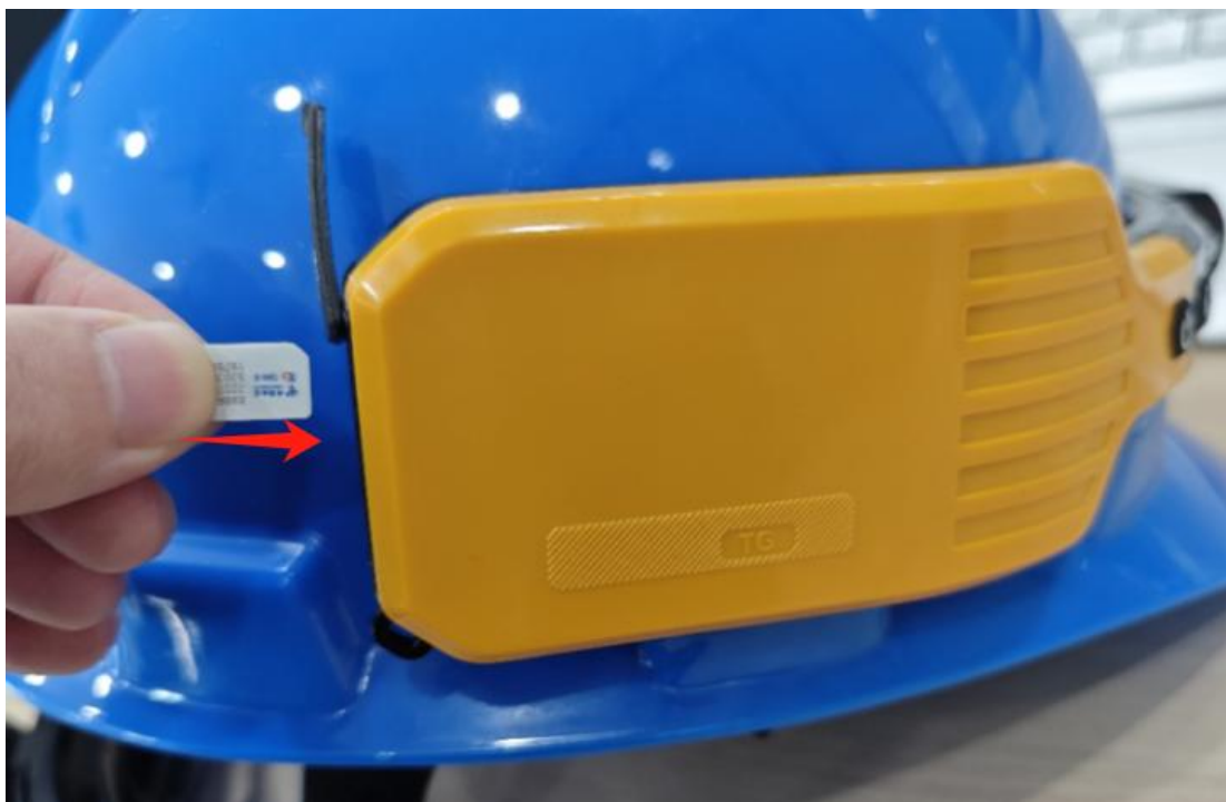
EQ-D6(HB) SIM Slot Insertion Diagram
