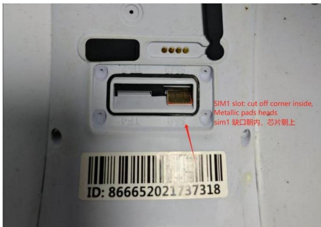
EQ-D6 SIM1 Slot Insertion Diagram
