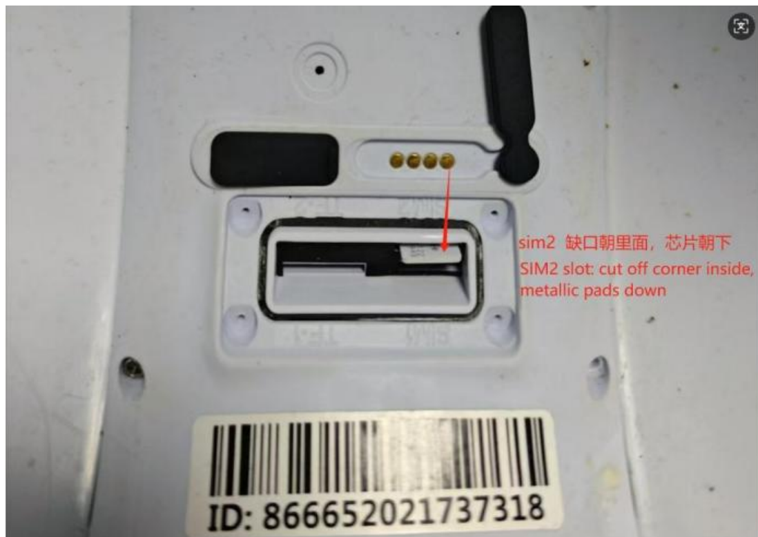
EQ-D6 SIM2 Slot Insertion Diagram
