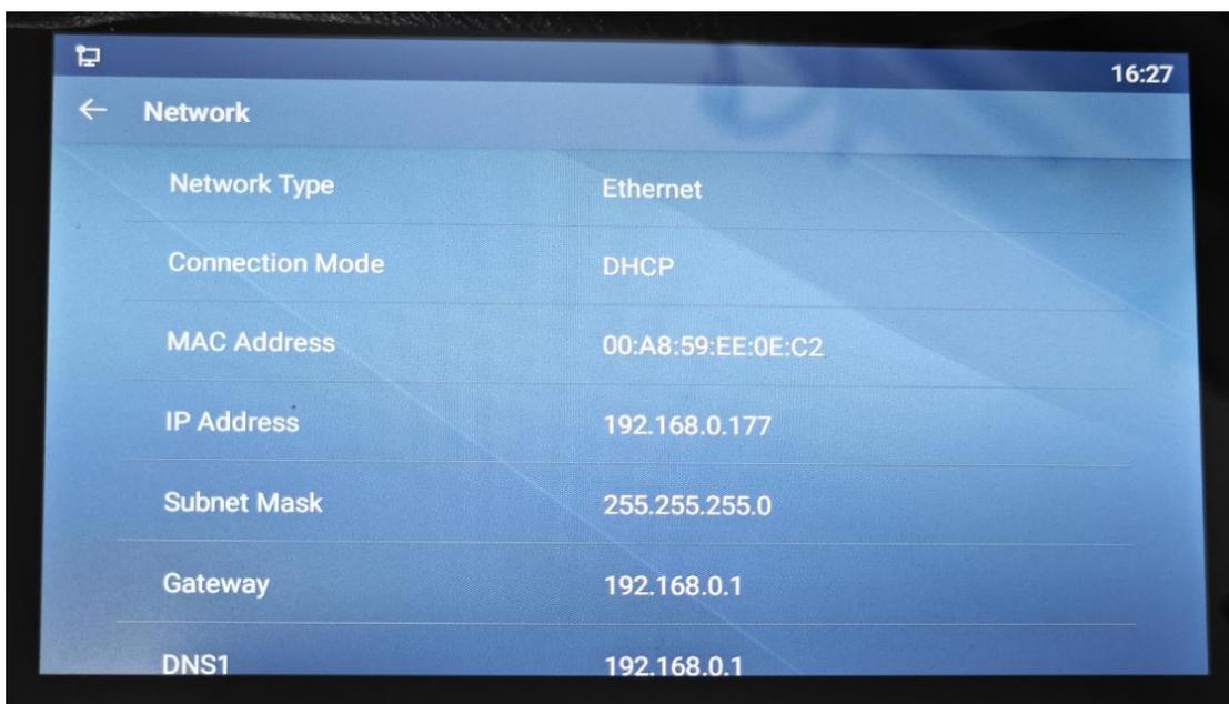
Without DHCP, unable to get a IP. We should set a IP manually. Go to Phone Settings>Ethernet, change the Network mode to Static, modify the IP and click on save.
