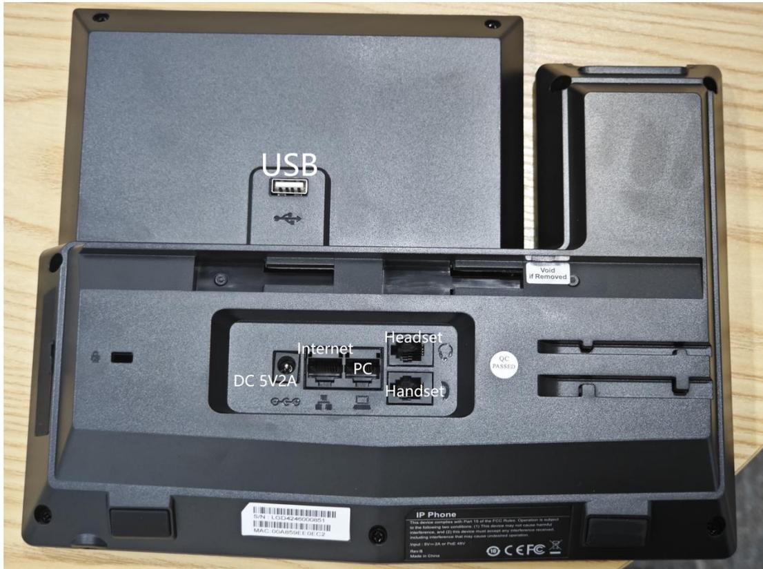
2. If connect to a POE Switch with DHCP, go to Phone Settings>Network to check the IP.
