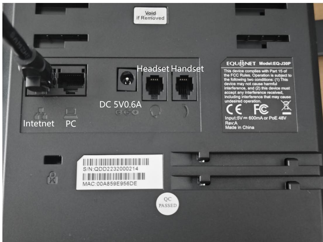
2. If connect to a POE Switch with DHCP, go to Menu>Status to check the IP.
