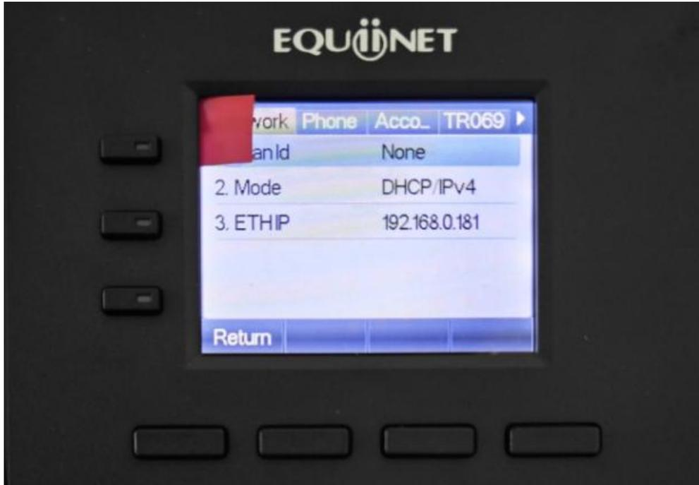
**Without DHCP, unable to get a IP.** We should set a IP manually. Go to **Menu>System(password:123)>Network>Network>IPv4**, change the Network mode to Static, fill in your IP.
